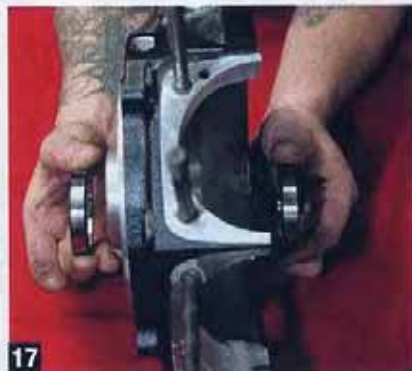
17 Next, a pair of bearing races needed to be pressed into the left side case, sandwiching the snap ring.
