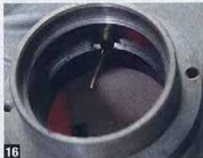
16 A good look at the snap ring in place with the gap positioned at the top ensures proper oil flow to the bearings. To demonstrate the direction of the oil flow, Eric inserted a pick in the oil passage drilled in the case.
