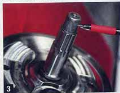
The sprocket shaft could be considered the business end of the flywheels, since it protrudes through the left case half and into the primary as it drives the compensator, sprocket, primary chain, and clutch. ▶
