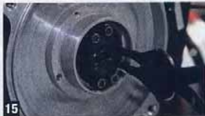
15 ...but the snap ring must first be installed in the left-side case half with this slick little tool made by JIMS (part No. 1710). Without this tool, installation would be very difficult, and damage to the case is a distinct possibility.
