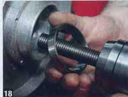
18 This custom-made tool makes race installation a breeze. ▶
