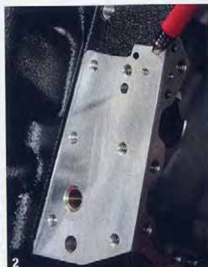
Further inspection showed that the same care had been taken in the oil-pump mounting area, as well as in the other surfaces.
