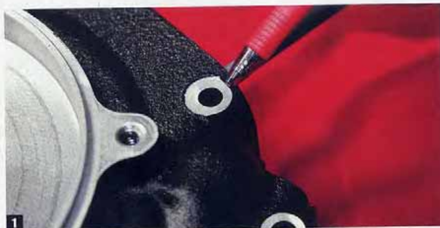
Before beginning, we inspected the cases and were impressed by the care taken at Concept Powder Coating to meticulously mask off all the areas where the washers would sit under the case bolts.
