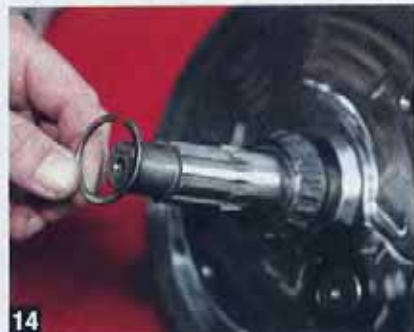
14 ...readying the outer race snap ring for installation. The sprocket shaft will eventually pass through the outer race snap ring...
