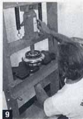
The stock hub was then carefully pressed out of the clutch basket with the help of a hydraulic press. ▶
