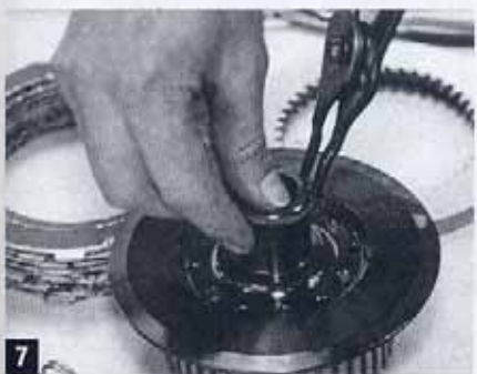
7 Since we were reusing the stock Harley clutch basket, Eric Bennett disassembled the clutch assembly, making sure to remove the new snap ring installed on the hub.
