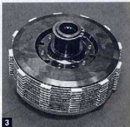
The backside of the assembly reveals the splined bore that will interface with the transmission's mainshaft.
