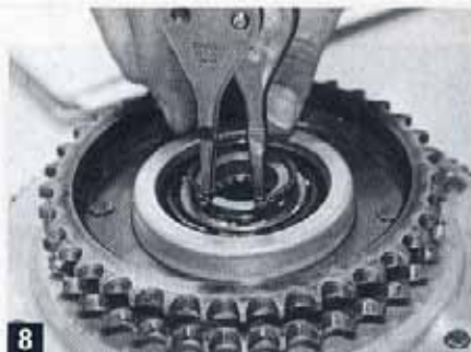
8 He then removed the snap ring from the stock clutch hub on the backside of the clutch basket.
