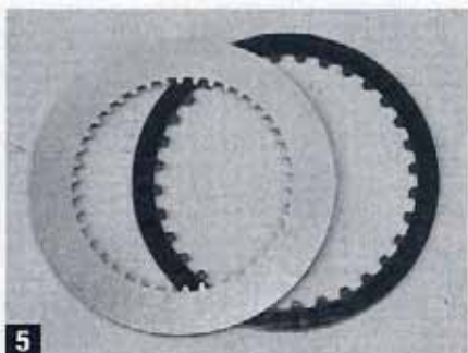
5 The same goes for the steel drive plates. All told, the Scorpion will give you approximately 100-percent more gripping surface than the stock clutch. This extra area allows for the use of lighter clutch springs without the fear of slippage.
